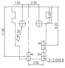
Recommended PCB Layout Top View
