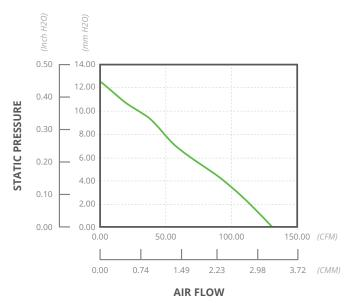
Next, the actual system impedance (previously characterized by system profiling) is overlaid on the fan performance graph and the point at which the curves intersect is the required system operating point (Figure 6).
