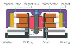
Ball bearings (Figure 2) do not suffer from the problems of uneven wear and friction associated with sleeve bearings, meaning they have a much longer operating life. They can also be operated at any angle, making them suitable for use in portable applications. However, they are less robust (vulnerable to sudden impacts), more complex, and costlier than sleeve bearings.
