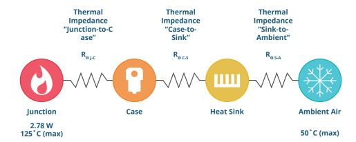
The "junction-to-case" thermal impedance is denoted by the symbol  $R\theta$  J-C and is used to quantify the amount of heat transferred from the silicon junction of the transistor to the surface of the package in which it is housed. Manufacturers typically list this impedance on the device datasheet, alongside the figure for junction-to-ambient impedance. The junction-to-case thermal impedance for the transistor used in this application is specified as  $0.5^{\circ}\text{C/W}$ .
