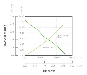
In systems where the airflow cannot be measured, an alternative approach is to specify the fan operating point to be above the idealized figure calculated from the equations. For example, if the required airflow is determined to be 50 CFM (in ideal conditions), a logical approach is to specify a fan with an airflow capacity up to 100 CFM. Operating the fan at 75 CFM provides 50% overhead
